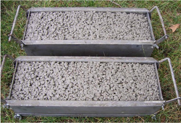
Figure 46. Fresh concrete with no curing compound
